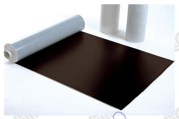
Renova UNO was developed for renovation projects, its one side is self-adhesive, and this product is a special polymer bituminous, polyester carrier, 3 mm thick. Especially in the roof insulation of historic structures which have fire risk, it has a characteristic of being implemented thanks to the fact that it is self adhesive without using torch flame.
